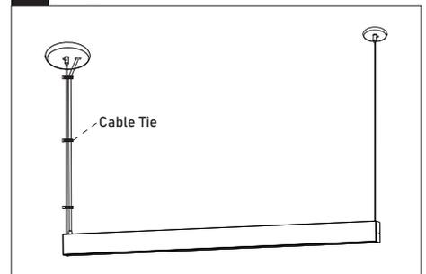
Use the cable tie to keep the electric wire going up along with the wire rope.
