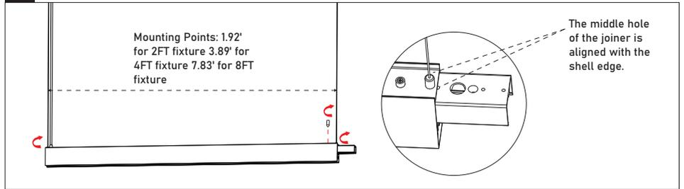
1-1:Screw both bottom parts of aircraft cables clockwise and secure them on the top of housing making sure they hang the lights.
