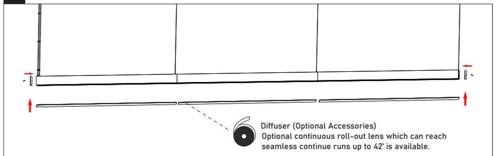
3-1: Reload the PC diffusers into the housing in turn. 3-2: Reload the end caps and fix with screws.
