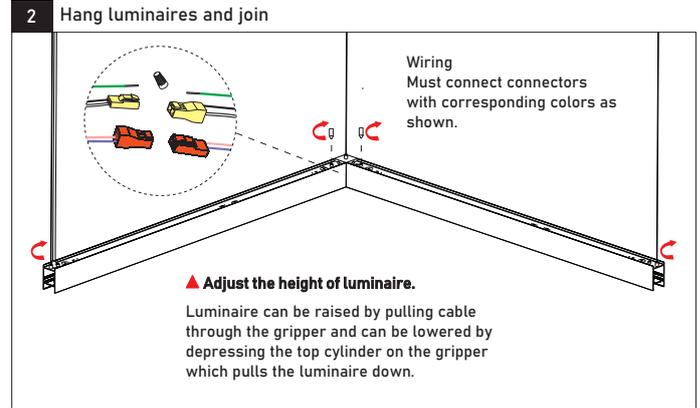
2-1: Screw aircraft cables clockwise and secure then , making sure they hang the lights. 2-2: Insert the joiner "L" into housing, and connect the quick connectors properly
