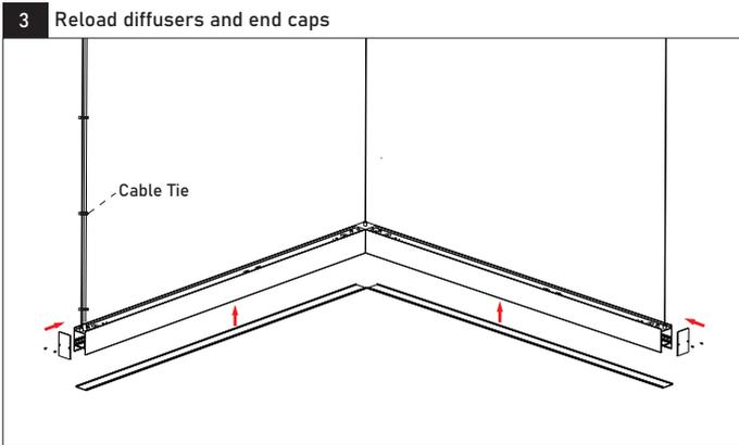
3-1: Zip tight power cord & aircraft suspension cable with the cable tie.
