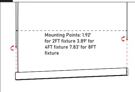
Screw both bottom parts of aircraft cables clockwise and secure then on the top of housing making sure they hang the lights.
