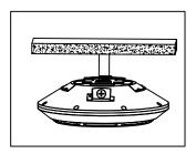
3.Attach the Canopy light with bracket by putting the ring on clips again. Connect the Black wire for line, white for Neutral, Yellow Green for Ground.
