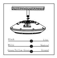
2.Fix the bracket on J-box ,and put the wire through the central hole for wiring
