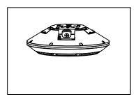
4.Slide the Canopy lights into bracket, and secure the screw on side of the light to prevent the light sliding out from the bracket. Installation done.
