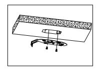
3. Screw the conduit into the hole on top of canopy light. Installation done.
