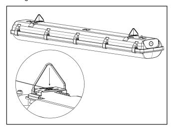
3.Hang fixture from customer supplied chain using V-brackets.
