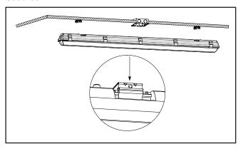
4. Without touching LED boards, detach LED tray and lens from fixture.
