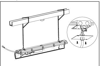
9. Secure lens to housing with lens latches.
