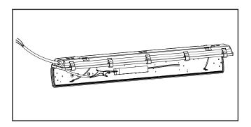
Secure mounting clips to housing recesses by firmly pressing them into place until both sides of the clip are secured.
