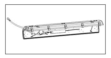
8.Reattach LED tray and lens to fixture by reversing step 5.
