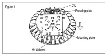
3.Connect the clip on the fixture to the spindle of the mounting plate to make sure the fixture will not slip and fall.connect the line voltage to the wires coming out from the fixture following the wiring diagram.Push the pressing plate into the suspension loop on the mounting plate.
