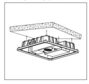
Remove 1/2" plug from direction you intend to feed conduit.
