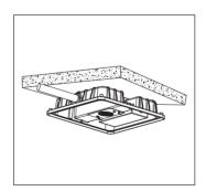
4. Disconnect the wires came from 3/4" hole and connect the wires came from 1/2" conduit with canopy . (White for Neutral, Black for Line, Green/Yellow Green for Ground)
