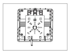
2. Connect the wires threaded from conduit and Canopy, Black wire for Line, White for Neutral, Green/Yellow Green for Ground.
