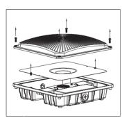
2.Cut off the wires through from 3/4" hole and plug the hole with provided Plug. Drill 4 holes on edge of fixture and fix it on the ceiling with using appropriate screws.
