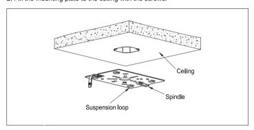
4. lock the M4 screws to complete the intallation.
