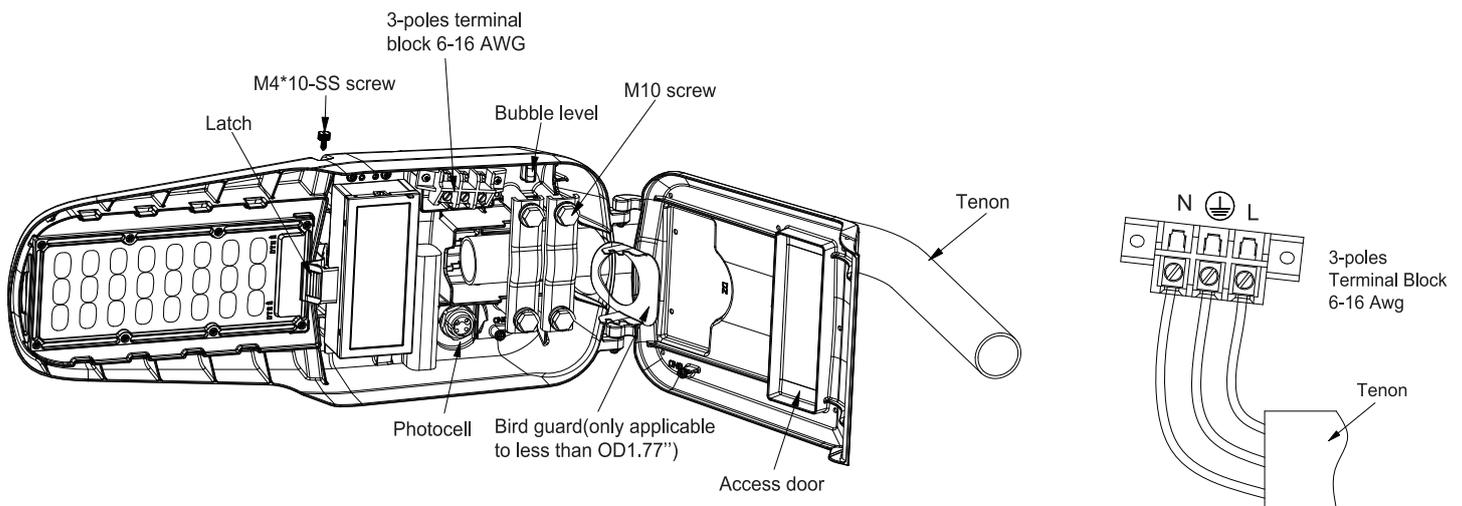
Horizontal angle can be adjusted in 2.5° steps, ±5°
