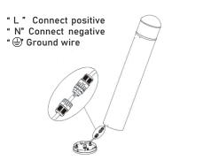
4. Through the waterproof connector on the power supply, connect the wire as required and tighten it; As shown in the picture above:
