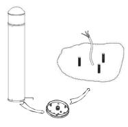
2. Disassemble the base of the lamp and use the holes of the base to locate the accurate position of the three tooth rods; As shown in the picture above:
