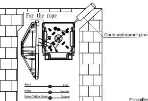
2) Fix the cover of driver and waterproof cotton pad on the wall.
