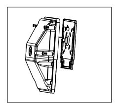
3) .After installation, daub the gap between installation board and wall by waterproof glue to avoid leaking, Hang the rope to cover of driver to avoid falling. And connect AC wire.
