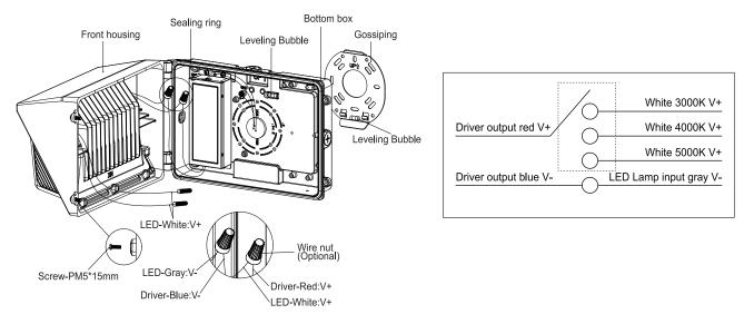
2. Make sure that all wires are securely connected and that there are no exposed conductors. Cover the fixture, (Make sure wires do not get pinched) then tighten the screws.
