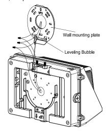
Note: To ensure waterproof seal, apply weatherproof silicone sealantaround the edge of the wall mounting box and /or junction box.
