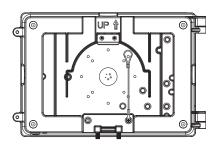
Stick EVA gaskets on the back of the wall mounting plate properly, which is very important for water proof.
