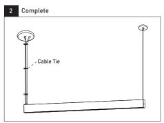
Use the cable tie to keep the electric wire going up along with the wire rope.
