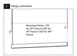
Screw both bottom parts of aircraft cables clockwise and secure then on the top of housing making sure they hang the lights.
