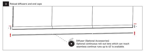
3-1: Reload the PC diffusers into the housing in turn. 3-2: Reload the end caps and fix with screws.
